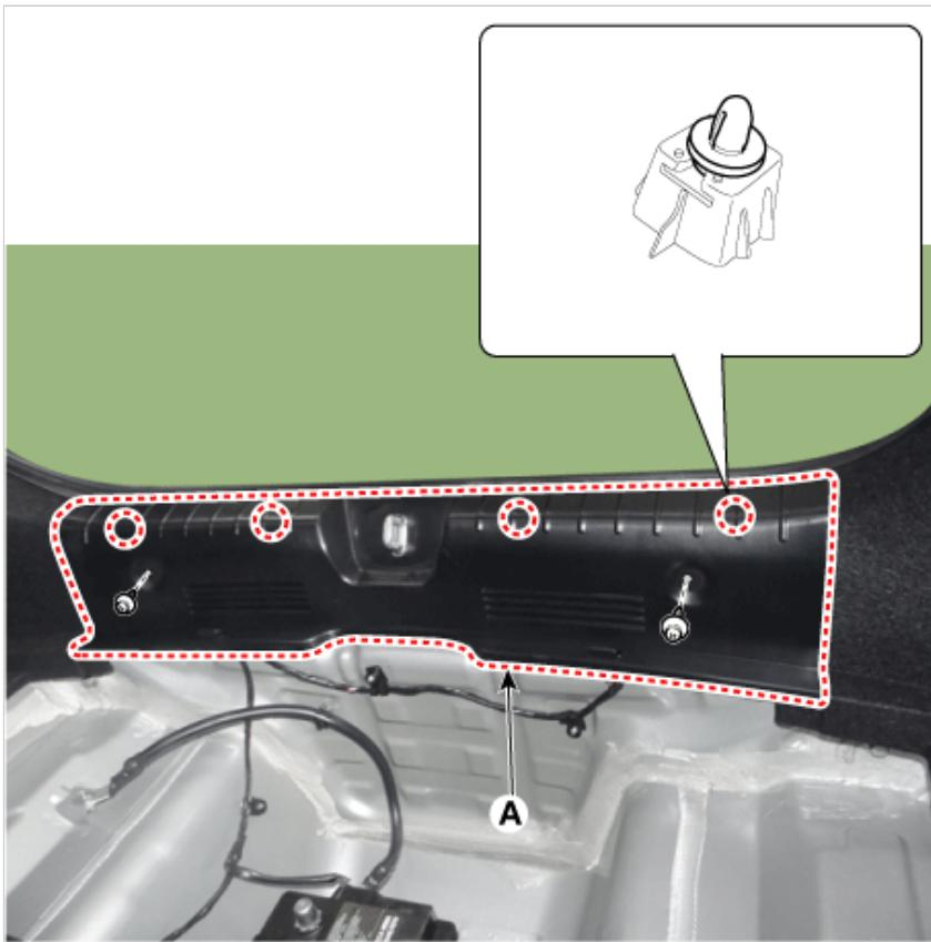
12. Separate the luggage side trim (A) after loosening the mounting screws.
