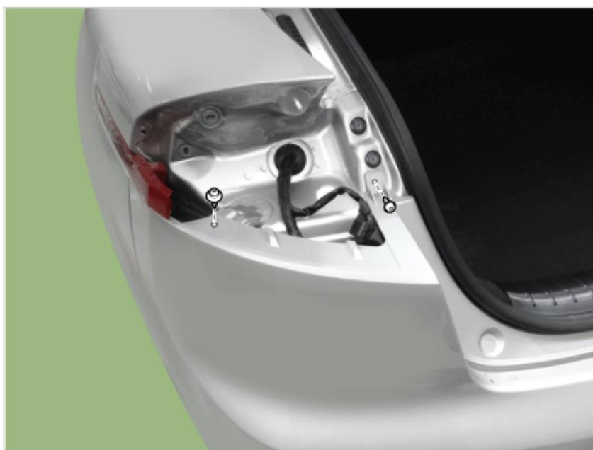
7. Remove the rear bumper side under cover (A) after loosening the mounting nuts and clips.
