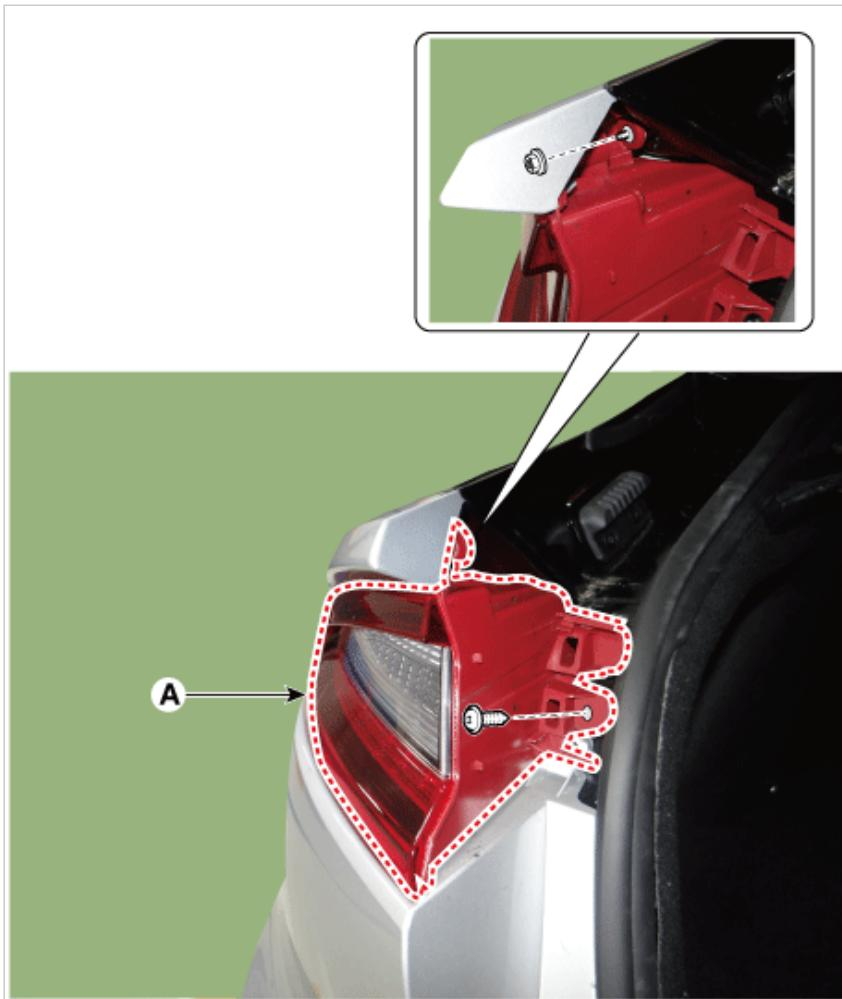
4. Disconnect the rear combination lamp connector (A).
