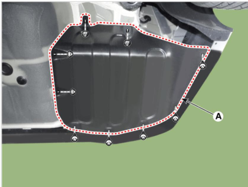
8. Separate the bumper (A) side after loosening the mounting screws and clip.
